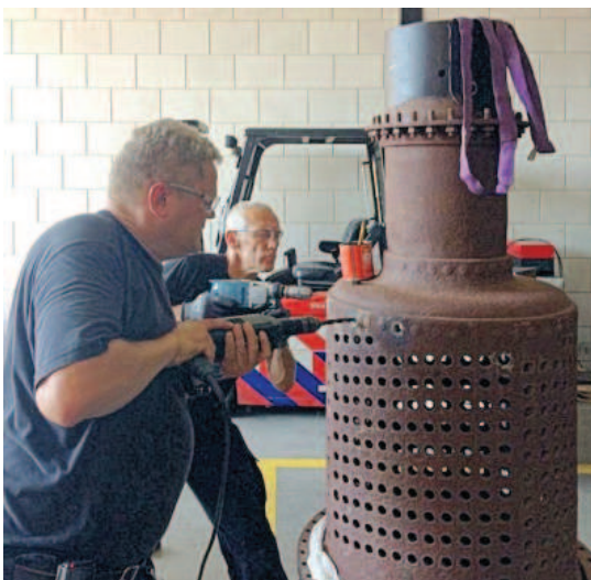
Drilling out rivets from the Shand Mason boiler of Cerberus.
